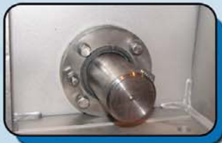
Stuffing Box Seals Provides blow-out protection
